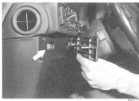
Fig. 12. Lower instrument panel trim cover being removed on cars with SRS airbag. Pry cover out of clip (arrow), then slide cover outwards toward left.
