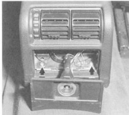
Fig. 1. Center console mounting screws at rear of console (arrows).
