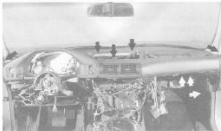
Fig. 7. Instrument panel mounting screws (arrows).
