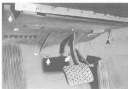
Fig. 13. Pedal cluster trim panel retaining clips (turn 90° to release) and mounting screw (arrows). Retaining hook is located at A.
