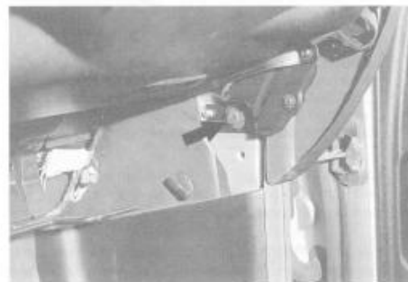
Fig. 10. Mounting bolt at lower right side of instrument panel.
